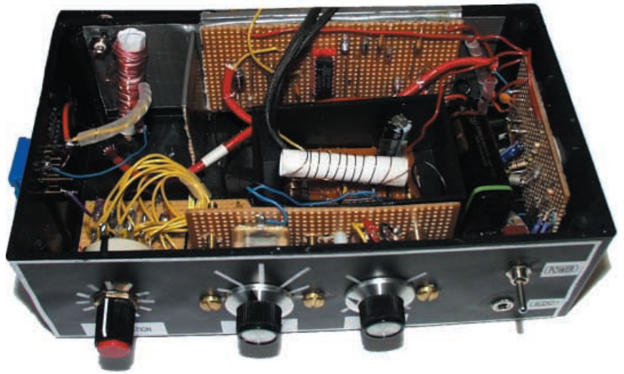
Positioning of the circuit boards and L1/L2 inside the case. The Tuning board is mounted inside its own potting box. Note the small “screening” partition by L1/L2.
